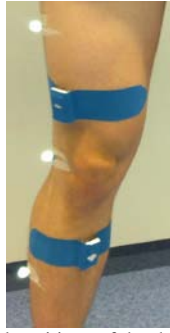
Fig. 1. Recommended positions of the thigh and shank sensors
